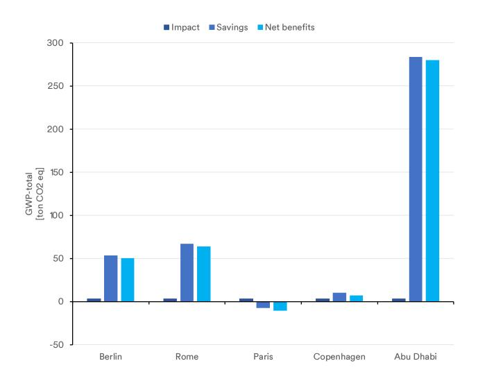
The second part of the analysis shows the GWP-total when a break-even point is reached and potential environmental net benefits are generated for the remaining lifetime of the film.
