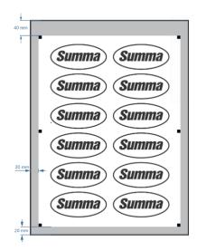
FIG 3-2 MARGINS PRINTING ON A SHEET
