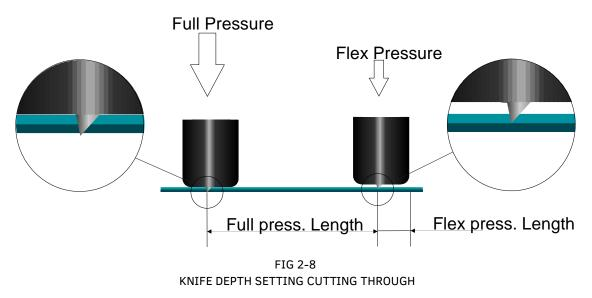
When performing FlexCut the knife is turned out just enough to cut through the vinyl and backing. The decision to let the knife holder rest on the media at full pressure depends on the actual media you are using. If the media is prone to scratching, then make sure the bottom of the knife holder does not touch the media when using full pressure. If not, it is recommended to let the bottom of the knife holder touch the media at full pressure.
