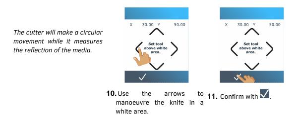
The cutter will make a circular movement while it measures the reflection of the mark colour. Then it will show a value that is characteristic of this media colour – mark colour combination. Store this value for future reference.
