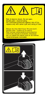
Fuse caution label. For continued protection against the risk of fire, replace the fuse only with the same type and rating of the fuse.
