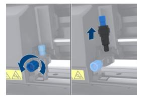
FIG 1-13 REMOVING THE DRAG KNIFE HOLDER FROM THE CLAMP
