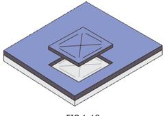
FIG 1-18 PEELED KNIFE PRESSURE TEST PATTERN
