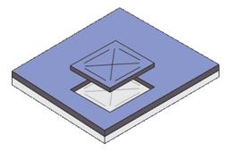
FIG 2-3 PEELED KNIFE PRESSURE TEST PATTERN
