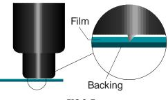
FIG 2-7 KNIFE DEPTH SETTING NORMAL CUTTING
