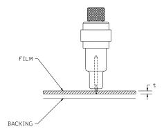
FIG 1-15 KNIFE LENGTH ADJUSTMENT
